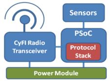
Fig.1. Blocks of wireless sensor node
